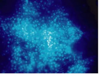
Digital photomicrograph of archael biofilm fragment in ground water downgradient of a DBB treatment zone. Epi-fluorescence light microscopy with DAPI staining. Field of view ± 3,000 um<sup>2</sup>.
